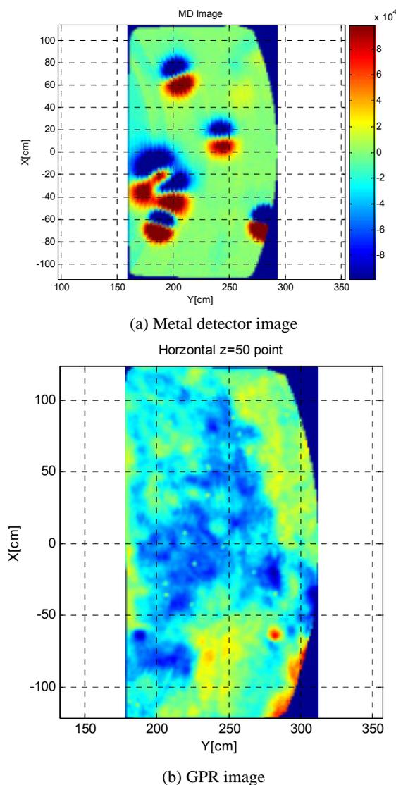
Fig.10 GPR image acquired by a buggy mounted ALIS
