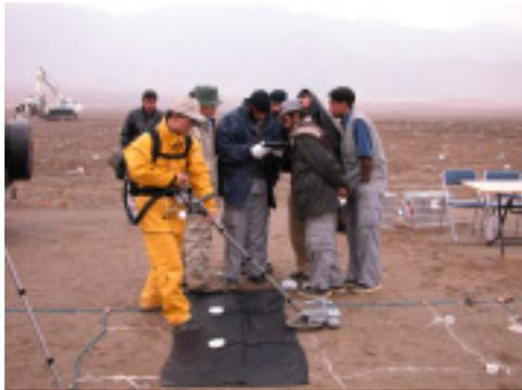
Fig.1 ALIS system under test at the CDS site in Afghanistan.
