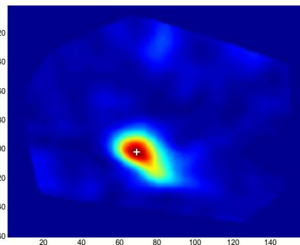
(b) Detected landmine in a horizontal slice.
