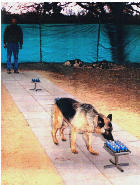
Figure 6: Checking vapour filters at a dog centre (V. Joynt, MECHEM)
