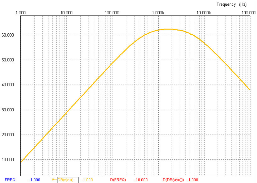
Figure 6 - Amplifier frequency response from 1 Hz to 100 kHz
